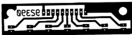
FIGURE 4-29. 81423 BANDSWITCH LED BOARD CIRCUIT TRACE
